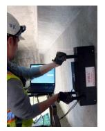
Once confident in the system's performance, WJE engineers used MIRA to scan a combined 319 feet of the bridges over a two-week period. Where voids were detected, discreet holes were drilled, allowing the engineers to perform borescope inspections of the offending tendon ducts. The engineers also excavated five inspection openings to verify MIRA results and collect grout samples for further laboratory studies. Despite the identification of eight grout voids, no tendon corrosion was observed.
